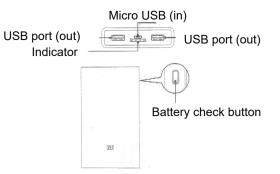
Note: the «battery check» button are not intended to turn on / off the device. This battery has the function of automatic detection of charging and discharging, so there is no need to constantly press the charge check button. In two minutes before the discharge, the amount of power LEDs are switched
